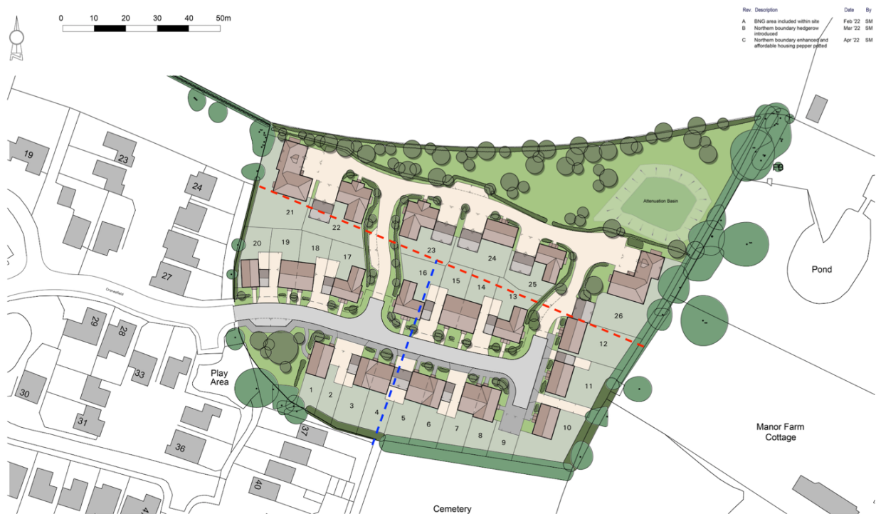
Fig 2: Submitted illustrative layout, produced by Sigma Planning Services (red dashed line added by ET Planning to show established building line, and blue line to show edge of low density area
